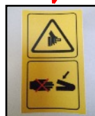
Danger of being crushed by moving parts
